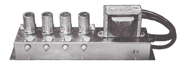
Model 1362 Bridging Amplifier has been designed for distribution applications at reasonable cost. Compactness and simplicity were also factors that dictated the final specifications.
