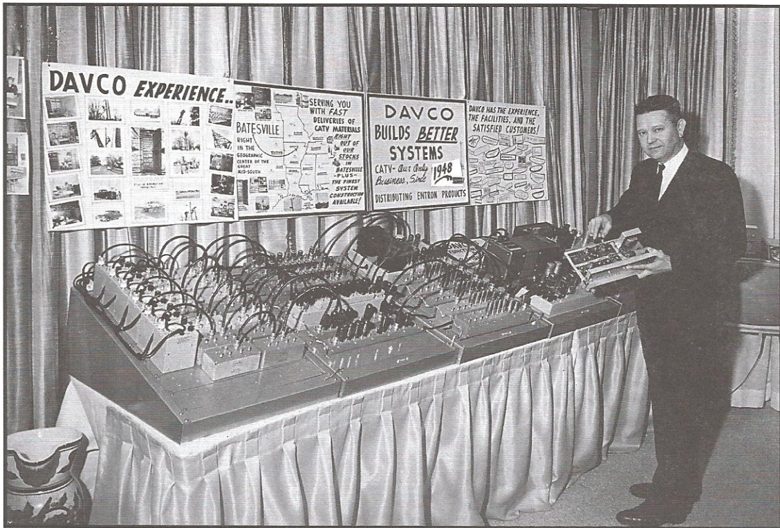
Jimmy Davidson, President of DAVCO Electronics, showing his "Functional Design" 12-channel head end at a cable convention in New Orleans in 1963
