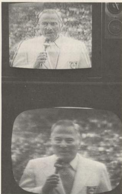
Photo Two — Bottom receiver still +10 dBmV; top receiver -10 dBmV.
