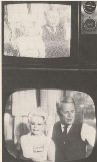
Photo Three — Bottom receiver +10 dBmV; top receiver -20 dBmV.
