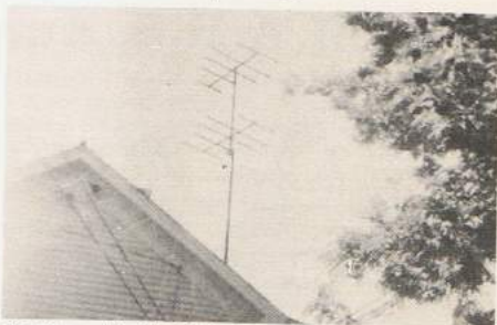
Ten-element Rotatable Yagi at Elving's Duluth home.
