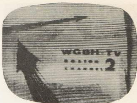
A good grade E skip signal from WGBH, Channel 2, Boston, as seen in Festus, Mo. by B. J. Bingham. Note the weak thin horizontal bars . . . more interference from a second Channel Two station.
