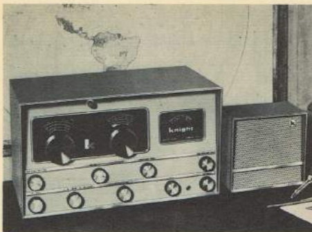
Allied Radio's Knight-Kit R-100 Receiver, with matching speaker. A well engineered and carefully planned general coverage receiver DXH recommends to even the novice builder.
