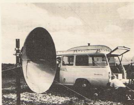
Adler Electronics field crew demonstrating UHF Translator operation to Laramie, Wyoming from a peak above town. Photo courtesy of Adler.
