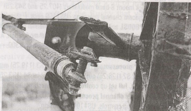
Two views of "what went first" - swaged (crimped) segment of azimuth movement pipe (at end of actuator) simply snapped in two freeing dish which wind whipped driving end of actuator through reflector surface destroying two panels.
